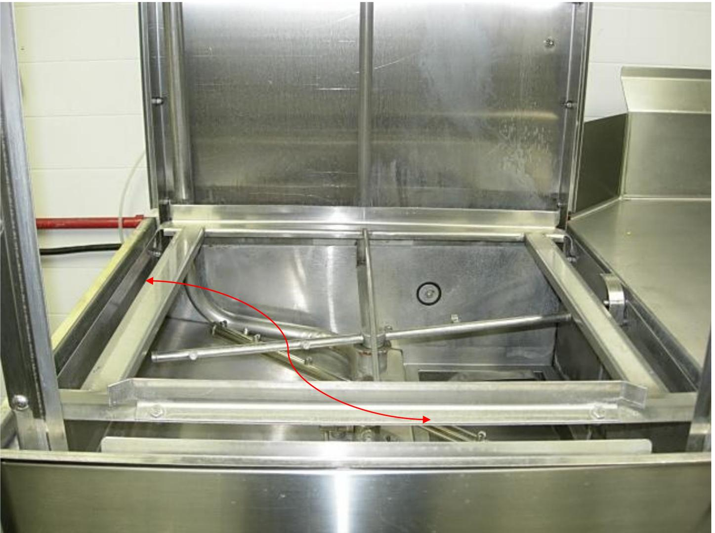
In order to convert machine from straight to corner application, you will need to relocate the tray track rail from straight to corner position (see red line on the photo) and then mount it on the tray track using the same bolts, washers and lock nuts used for straight application.
