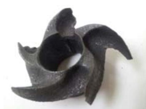
Impeller damaged from high acid solution
