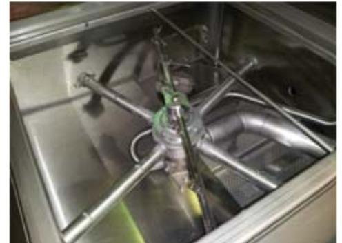
Final rinse arm twisted into transfer tube
