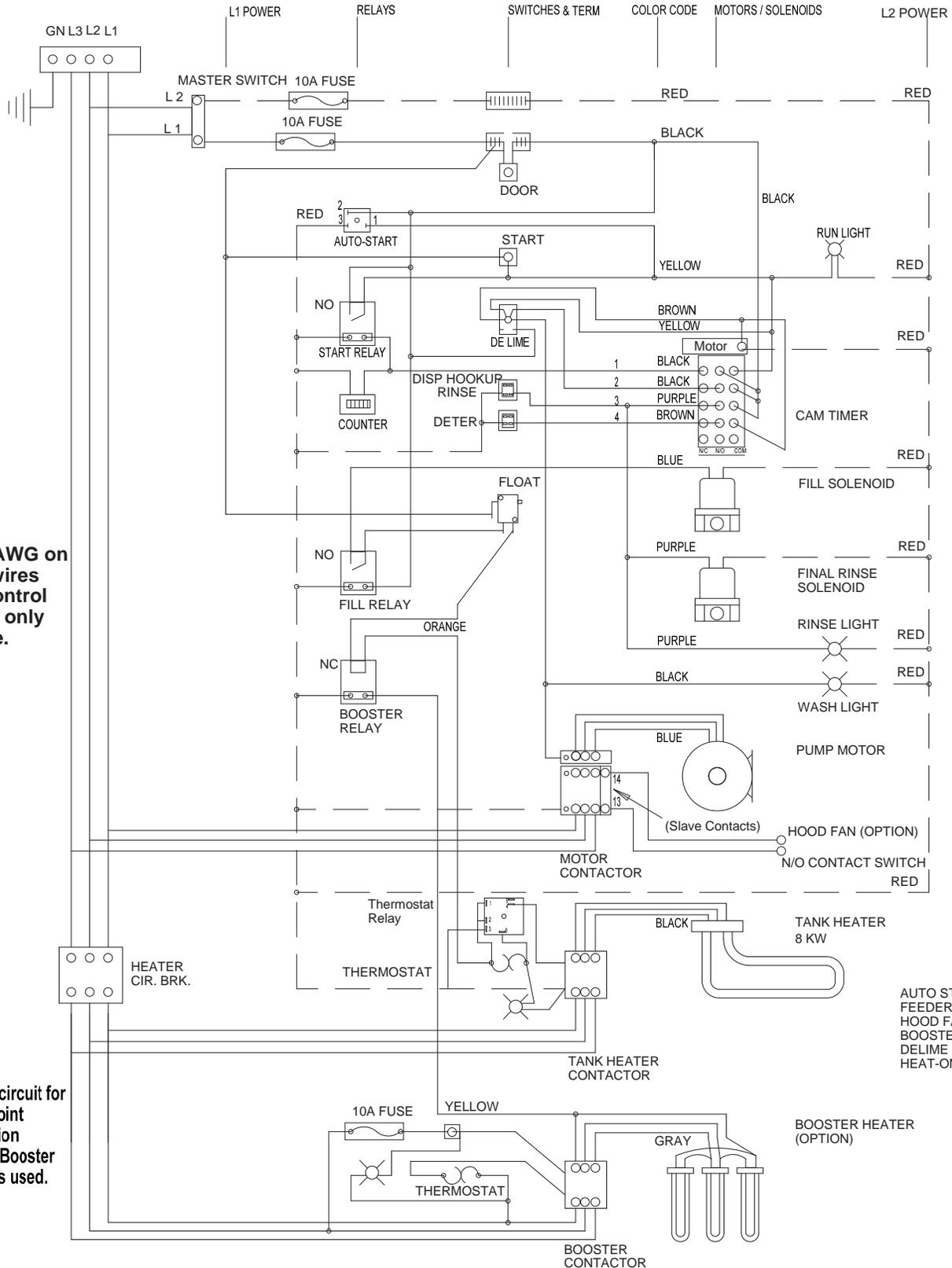
40 Amp, 8 AWG on L1, L2, L3 wires has 230v control circuit. Use only copper wire.
